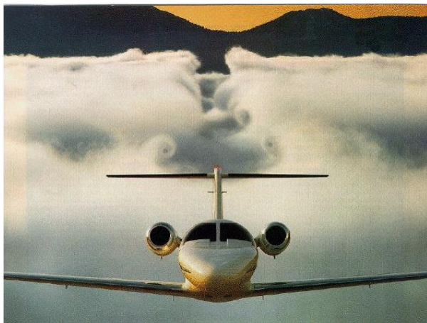
Figure 4-2 A good example of air being deflected downward as a jet flies over a cloudbank.
