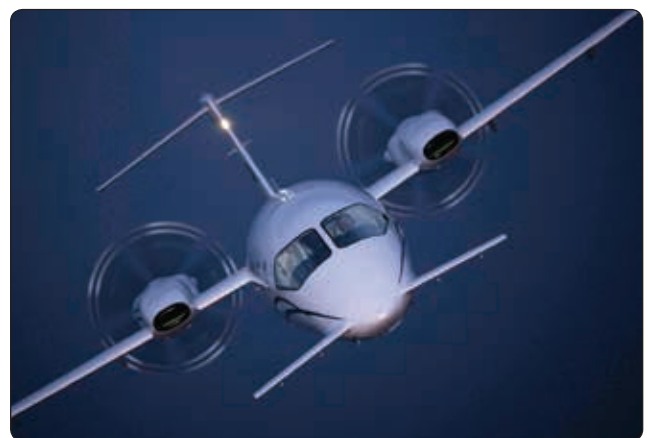
Figure 6-14. The Piaggio P180 includes a variable-sweep canard design that provides longitudinal stability about the lateral axis.
