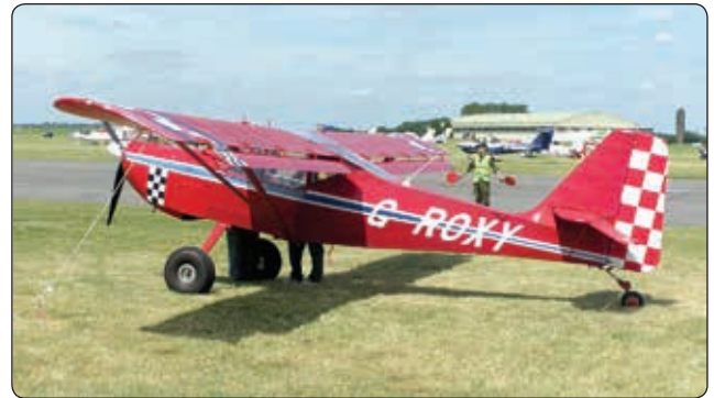
Figure 6-9. Flaperons on a Skystar Kitfox MK 7.
